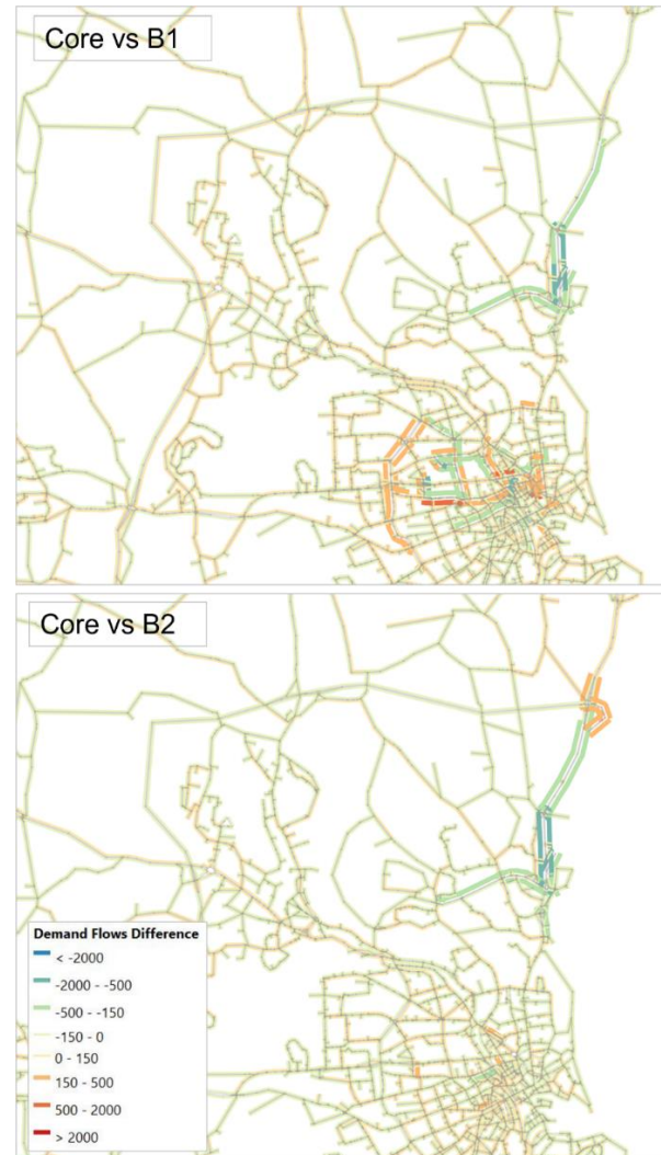
Figure 5.6: Road Traffic Demand Flow Changes (AADT) –Core Test vs Test B1 and Test B2
